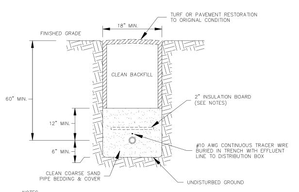
1. THE EXCAVATED TRENCH MATERIAL SHALL BE DEPOSITED AT THE SIDES OF THE TRENCHES AND USED FOR BACKFILL UNLESS DECLARED TO BE UNSUITABLE BY THE ENGINEED.
