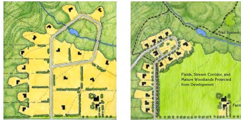
A comparison of a conventional subdivision (left) with a conservation subdivision (right). In both cases, a total of 16 residential lots are being created
