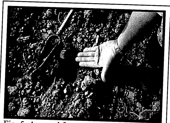
Fig. 5. Augered from a depth of 19 inches below the surface of the replaced topsoil, this subsoil sample was hand rolled to a 1/8-inch diameter. The test shows the soil at this site stretches out too far without crumbling; it indicates the material is in a plastic state of consistence, too wet for final decompaction (deep subsoiling) at this time.
