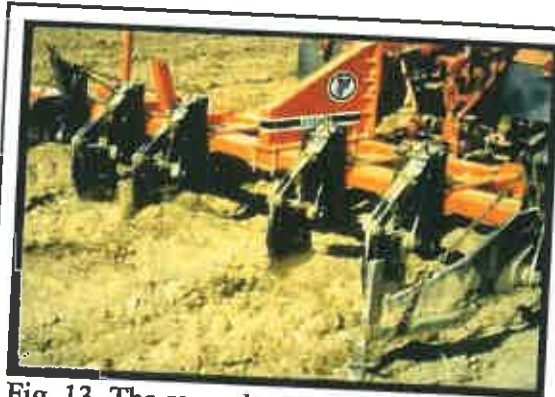
Fig. 13. The same deep, angled-leg subsoiler shown in Fig. 7 is engaged at maximum depth for Phase 2, decompaction (deep soiling), of the replaced topsoil and the upper subsoil materials.
